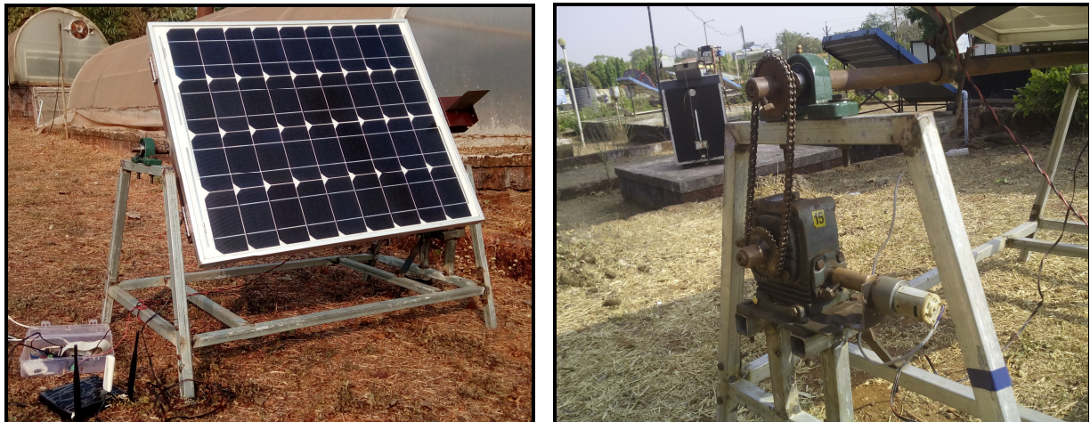
Fig11. Installation of Solar Tracker Unit on 80 watt photovoltaic panel
